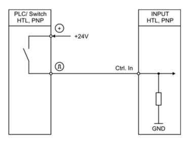
Unconnected control inputs are always "LOW". All inputs are designed to receive impulses from an electronic impulse source. Notice for mechanical switching contacts:
